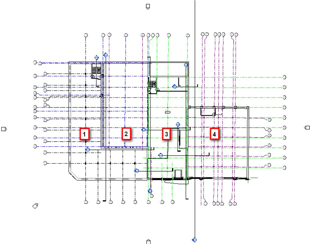
**Figure 1:** 210 King – Buildings 1 to 4 – grid lines. BLDG3 and BLDG4 grids are slightly askew
