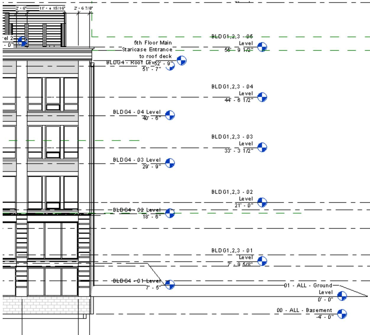
**Figure 2:** South elevation view showing the level heights for BLDGs 1 to 3 and BLDG4. BLDG4 levels are slightly lower than the rest.
