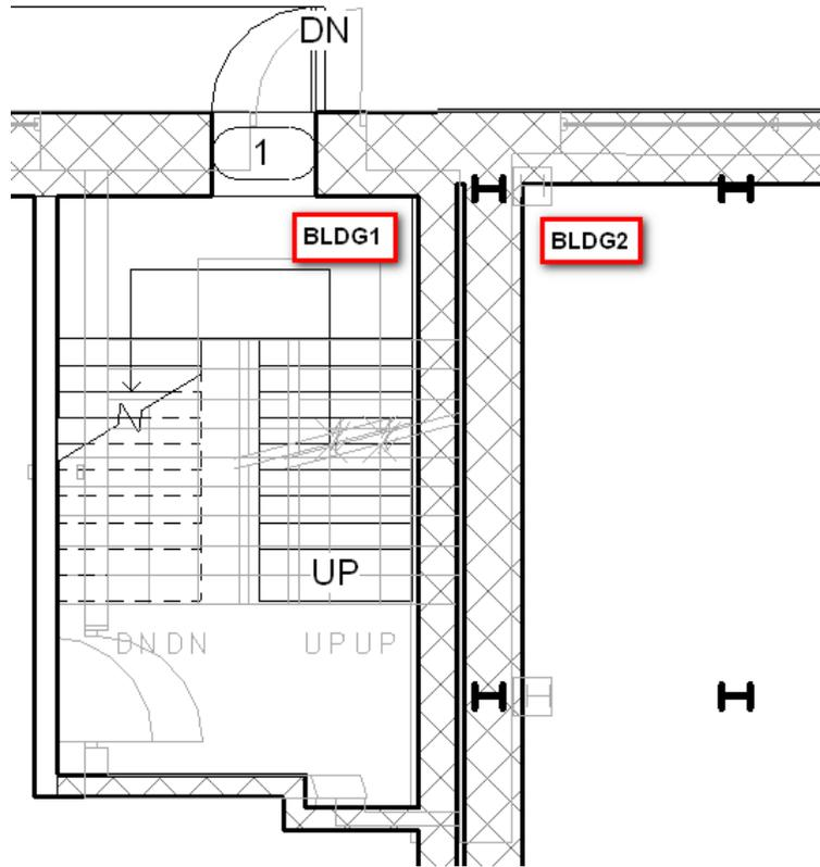
*Figure 3: BLDG1 and BLDG2 Adjacent foundation walls and exterior walls.*
